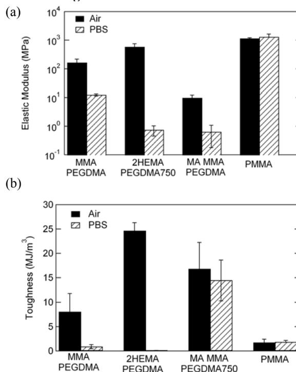
Figure 1. The effect of PBS on the elastic modulus (top) and toughness (bottom) of 3 acrylate-based networks and PMMA. Data are Mean<sub>±</sub>SEM.
