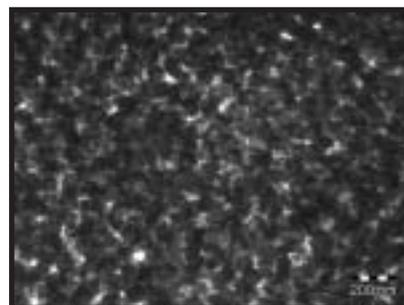
*Cover image 2: TEM image of a new dendritic SIBS-type biomaterial with 30 wt% polystyrene content.*
