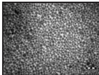
*Cover image 1: Transmission electron microscopy (TEM) image of a new dendritic polystyrene-polyisobutylene-polystyrene (SIBS)-type biomaterial with 9 wt% polystyrene content.*
